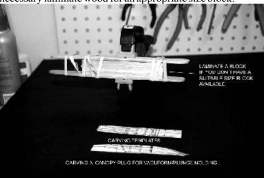
2. Cut out templates from the plan, or trace or copy the templates from the plan for laying out the canopy plug to be carved. Using the templates draw the outlines on the block. Reverse the templates for the opposite sides and mark top and bottom also.
