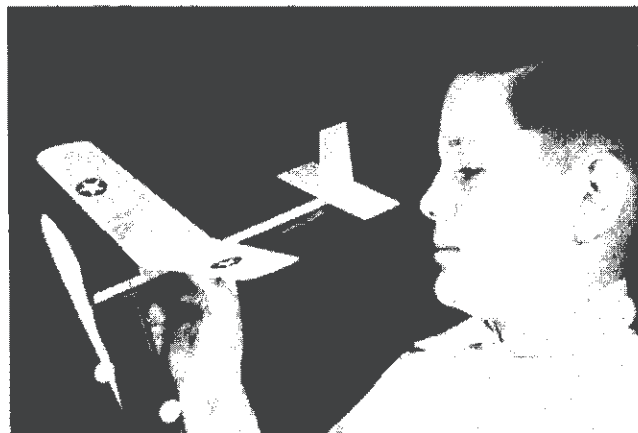
Junior here approves the whole idea. Rubber motor requires only two strands 1/8 inch rubber, nine inches long. No broken piggy banks for this.
