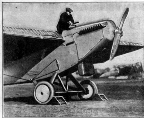
AIRFLOW VISUALIZATION USING SMOKE. In 1923, NACA Langley conducted one of the first in-flight flow visualization studies when smoke was trailed over the wings and control surfaces of a Martin MO-1, on loan from the Naval Air Station (NAS) Hampton Roads (now NAS Norfolk). The MO-1 was the U.S. Navy's first monoplane aircraft and made use of a thick metal wing for reinforced structural integrity, but it possessed several nagging deficiencies. During the flight investigations, the MO-1 was piloted by NACA test pilot Tom Cornell, while NACA Langley engineer David L. Bacon flew in the observer's position located in the midsection of the fuselage, photographing the smoke as it flowed over the wing. (NASA.)
